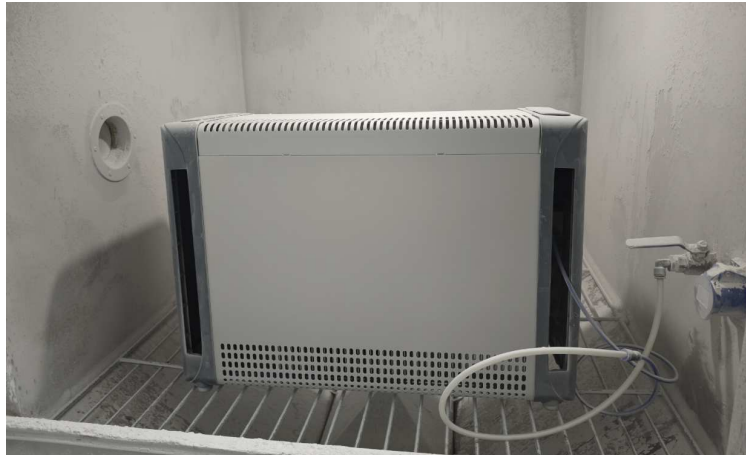
Test setup of IP6X
